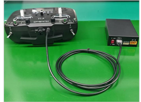
FPV ground setup: remote controller linked to the Ground Unit
