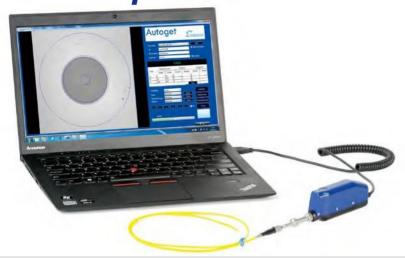
Autoget is an intelligent portable fiber enface inspector developed by PDR Videotronics Technology. It is equipped with newest hardware and software, and with functions of auto focus, auto exposure, auto analysis, auto generate report, auto image transmission, etc. 400X Autoget can detect the defects such dirts, scratches clearly by its software.
